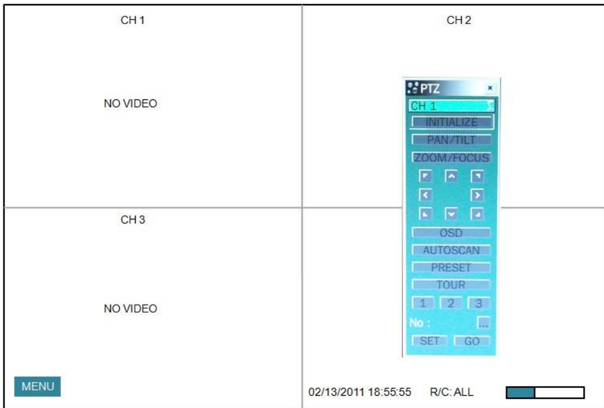
Figure 6.1.1. PTZ Control Screen
